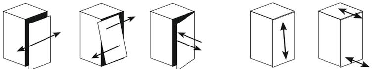
Horizontale, vertikale und axiale Justierung der Front. *The door position has three-way adjustment.*
